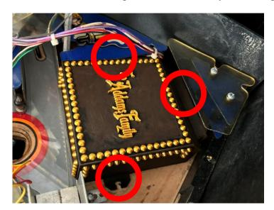
Slide the back in first then the top and adjust with the bottom screw.
